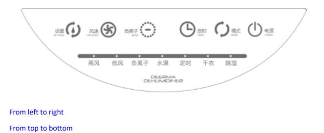
Setting Wind speed Negative ion Timing Mode power supply Strong wind Low wind Negative ion Full of water Timing Dry clothes Dehumidification
