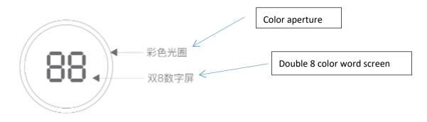
The display has a three-color aperture (red, blue, purple). After the machine is turned on, the aperture starts to light up. When the ambient humidity is above 70, it displays red; when the ambient temperature is below 50, it displays purple, and when the ambient humidity is 50-70 Blue is displayed between.
